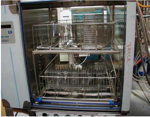
2 Level Wash Rack P/N 814456 includes: 6 – baskets – 820563 (see below) 6 – inserts – 820564 (see below)
