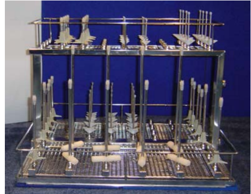
1½ Level Jet Rack - 835109 w/ 56 fixed jets (possible 30 add'l jets can be added)
