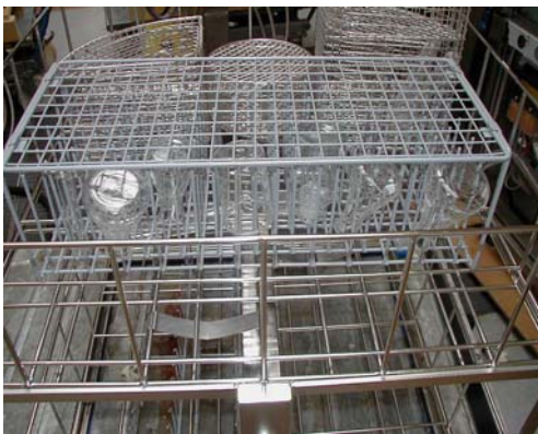
19" x 8" x 6" Baskets – P/N 820563. Accessories for 2 – Level Wash Rack. The baskets can be used with or without the inserts (P/N 820564)
