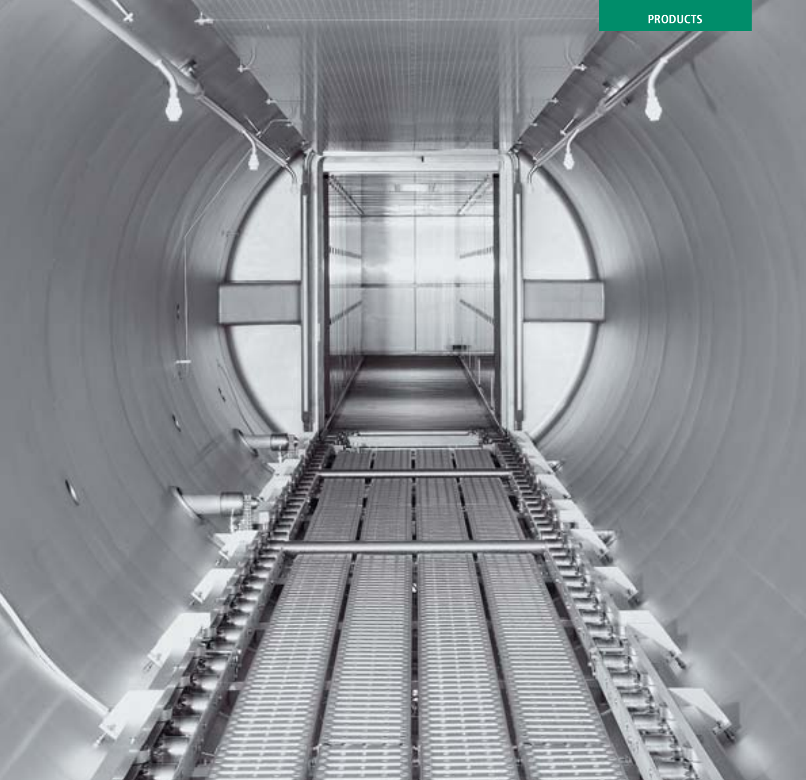
Internal view of a hot water shower steriliser with a chamber volume of 60 m 3 , automatic conveying, and CIP system
